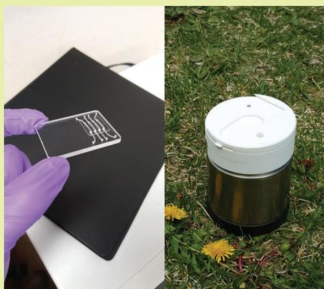
The test is housed in a thermos with a custom 3-D printed lid designed to hold a smartphone, which both activates and records the signal from the fluorescent dye. When colorimetric dye is used, the smartphone is not needed. The entire apparatus is inexpensive, and by switching the assays or tweaking the test to detect multiple diseases at once, it could be used to identify other pathogens.
