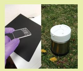
The test is housed in a thermos with a custom 3-D printed lid designed to hold a smartphone, which both activates and records the signal from the fluorescent dye. When colorimetric dye is used, the smartphone is not needed. The entire apparatus is inexpensive, and by switching the assays or tweaking the test to detect multiple diseases at once, it could be used to identify other pathogens.
